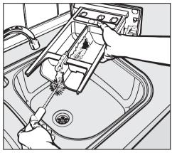
■ Remove the siphon from compartment \(\begin{align\*}\extre{\color{1}}\).
